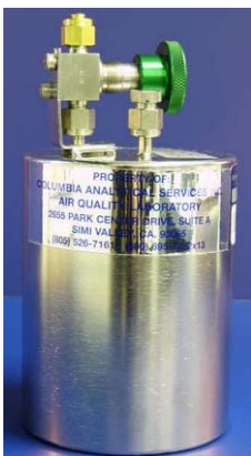
Figure 8. 1-L SUMMA canister for permanent gas composition.
